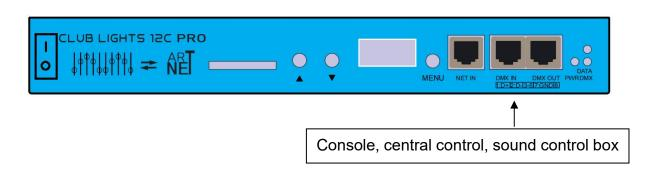
The external trigger command is a standard DMX512 signal, which is connected to an external DMX512 console and KTV intelligent lighting control box.
